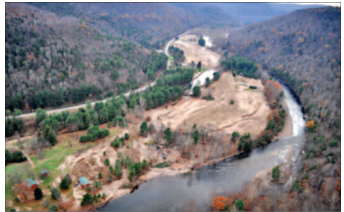
Berm breach near green-roofs and reconnection of channel to floodplain anabranches (Loyalsock Creek near Forksville).
