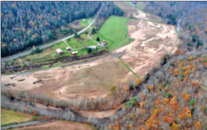
Chute across a farm, eroding multiple channels and depositing sand and gravel below berm breach (Muncy Creek).
