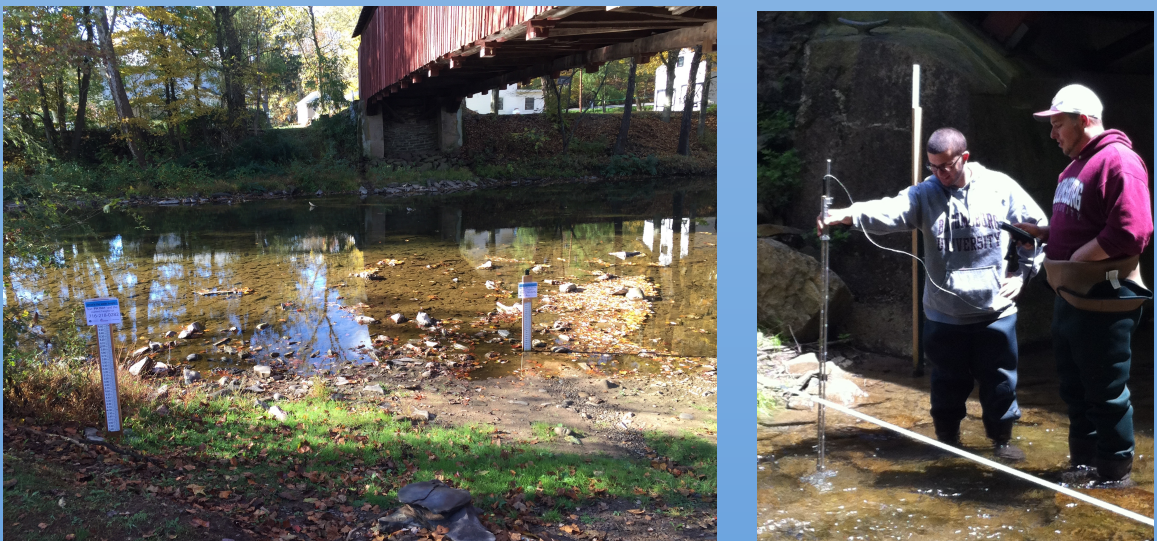
Figure 3. Stillwater Bridge gage site (left) and Shoemaker Bridge gage site (right), where Nate and Dereck are collecting a discharge measurement.
